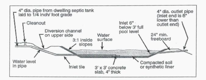
The lagoon banks should be at least 4 feet wide on top, with inner and outer bank slopes not steeper than 3:1. Freeboard of at least 18 inches, and preferably 24 inches, should be provided to prevent surface water from entering the lagoon.
